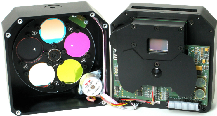
Illustration 20: Filters can be exchanged after removing of the camera front cover
