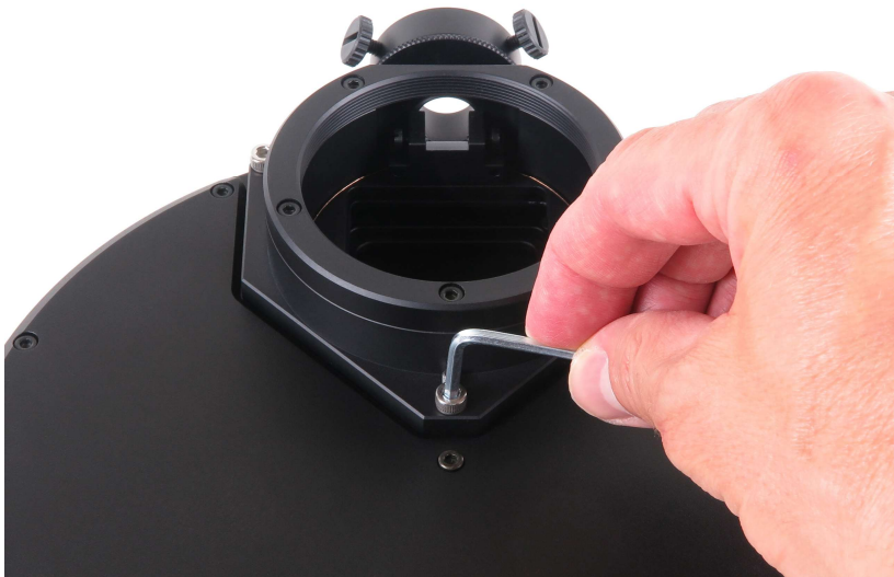
Figure 27: Adjusting of the "pulling" screw
