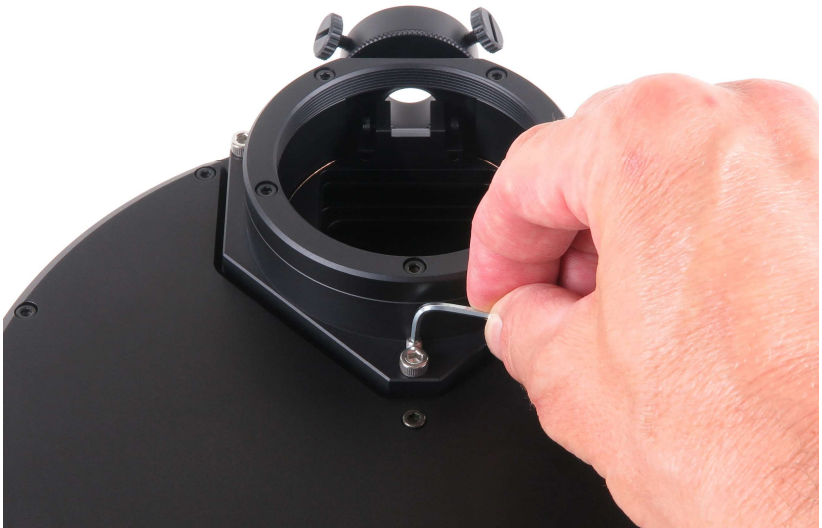
Figure 26: Releasing of the “pushing” screw
