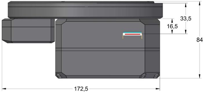
Figure 14: G2 camera head with External filter wheel side view dimensions
