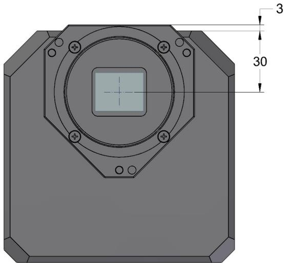
Figure 10: G2 camera head front view dimensions
