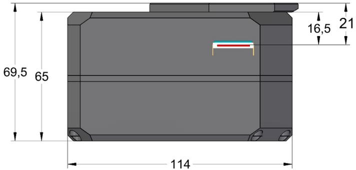
Figure 16: Camera without filter wheel with "thin" adapter base
