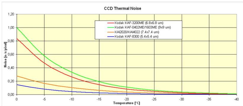
Figure 6: Dark current of some OnSemi CCD detectors, used in G2 cameras
