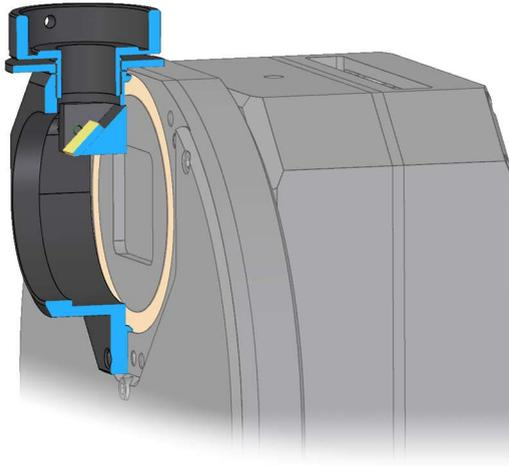
*Figure 19: G2-OAG sectional rendering illustrating reflecting mirror*
