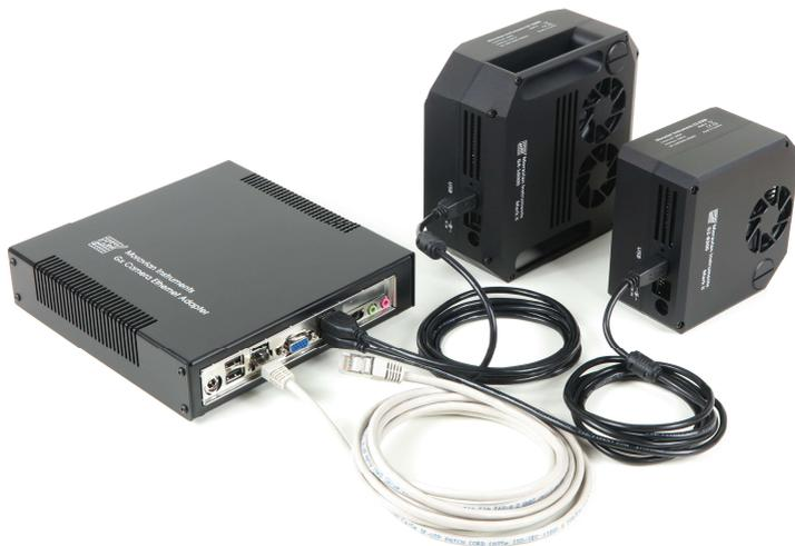
*Figure 22: The Gx Camera Ethernet Adapter with two connected cameras*
