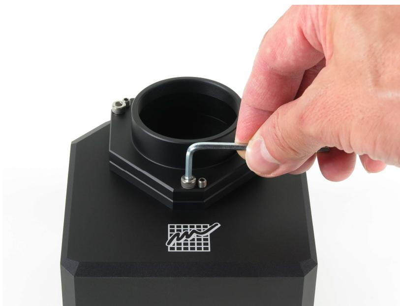
Figure 24: Adjusting of the "pulling" screw
