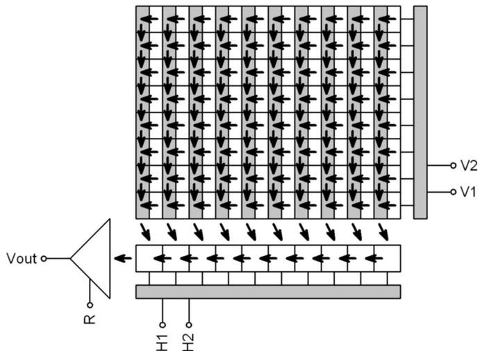
Figure 4: “Interline Transfer” CCD schematic diagram
