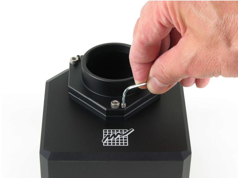
*Figure 23: Releasing of the “pushing” screw*
