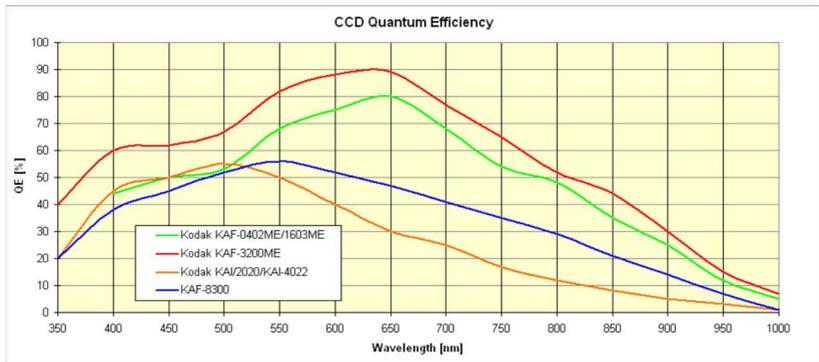
Figure 5: Quantum efficiency of OnSemi CCD detectors used in G2 cameras
