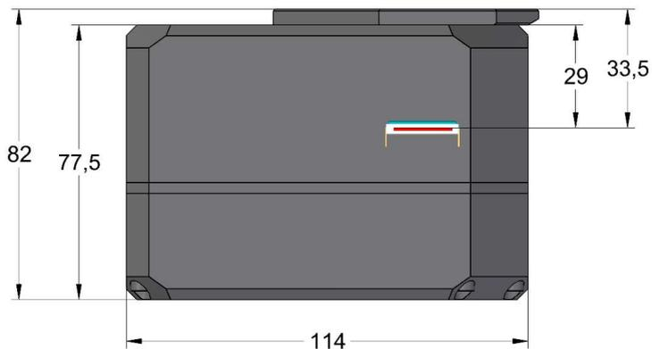
Figure 11: G2 camera head with Internal Filter Wheel side view dimensions
