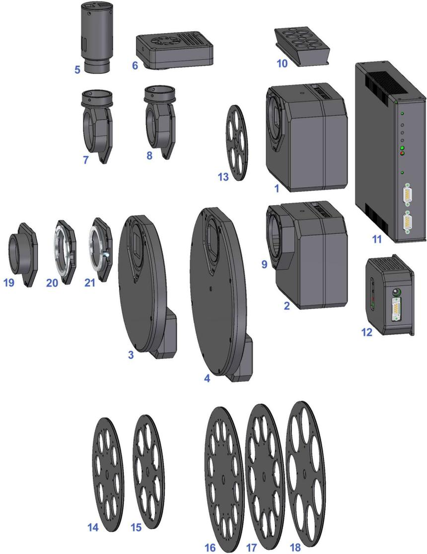
Figure 2: Schematic diagram of G2 camera system components
