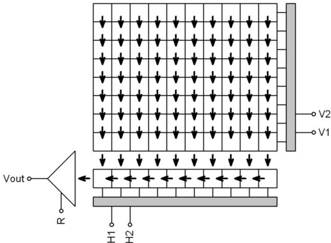
Figure 3: "Full Frame" CCD schematic diagram
