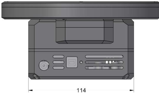
Figure 15: G2 camera head with External filter wheel bottom view dimensions
