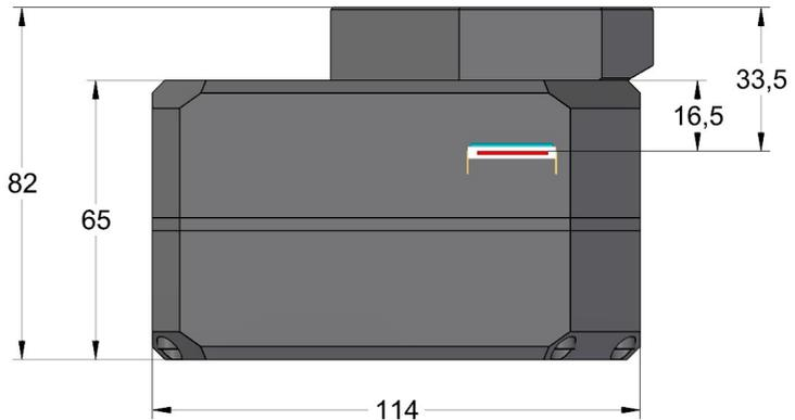
Figure 17: Camera without filter wheel with "thick" adapter base
