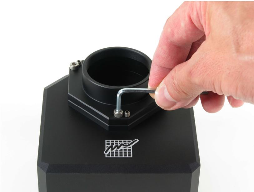
Figure 24: Adjusting of the "pulling" screw
