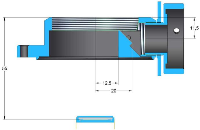
*Figure 18: Position of the OAG reflection mirror relative to optical axis*
