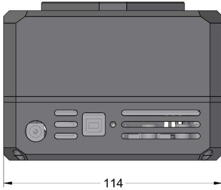
Figure 12: G2 camera head bottom view dimensions
