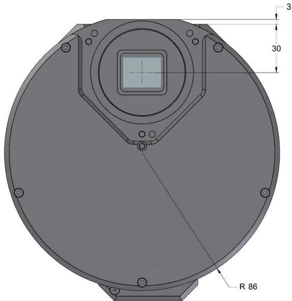
Figure 13: G2 camera head with External filter wheel front view dimensions
