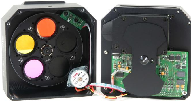
*Figure 29: Filters can be exchanged after removing of the camera front cover*
