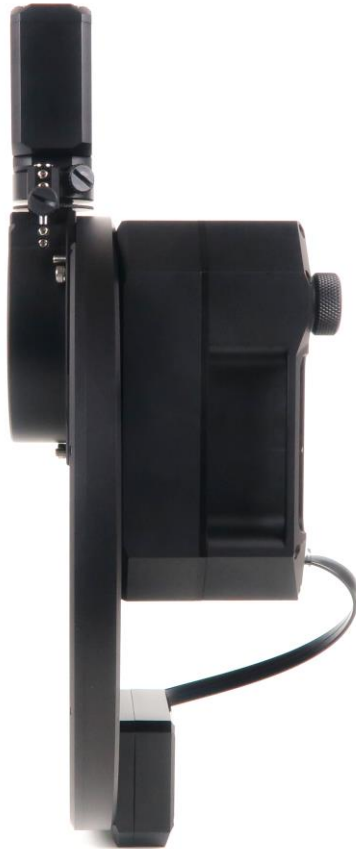
Figure 2: Side view of the C5 camera, SX-sized filter wheel, and C5-OAG adapter with attached CG camera
