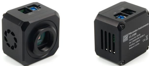
Figure 7: Cooling air intake is on the right side of the C1 camera (left image), while the output vents are on the opposite side (right image)
