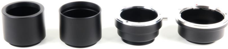
Figure 15: Extension tubes for C1 cameras with M42×0.75 adapter: T-thread with 55 mm BFD (far left), M48×0.75 thread with 55 mm BFD (left), Nikon bayonet (right) and Canon EOS bayonet (far right)
