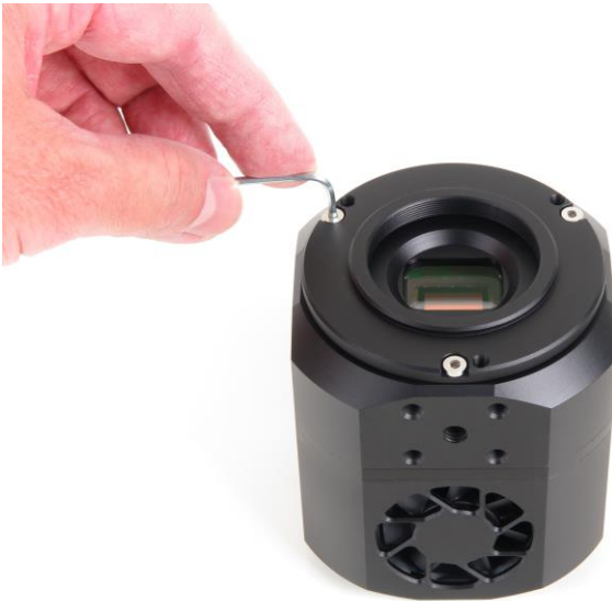
Figure 25: Adjusting of the "pulling" screw
