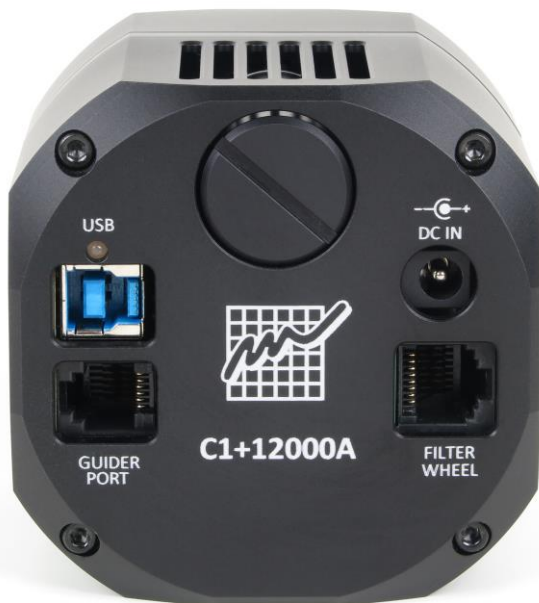
Figure 13: Standard 6-pin Autoguider Port is located close to the USB3 port on the back side of C1+ camera
