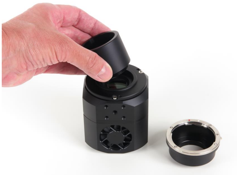
Figure 30: Replacing the C1 compatible telescope adapter
