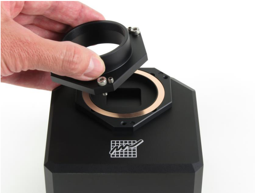
Figure 47: Removing of the adjustable telescope adapter
