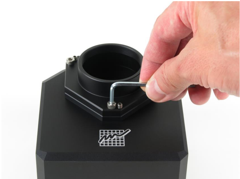
Figure 41: Adjusting of the "pulling" screw
