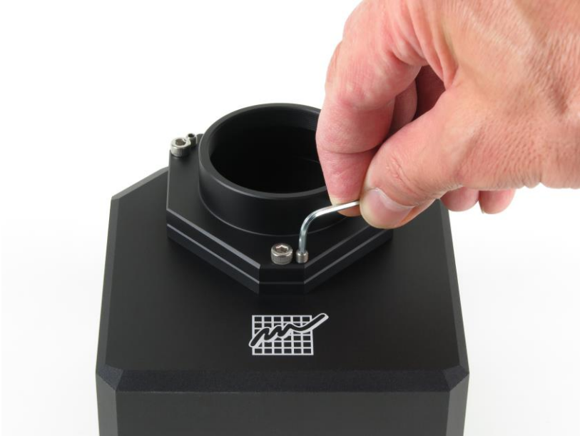
Figure 40: Releasing of the “pushing” screw
