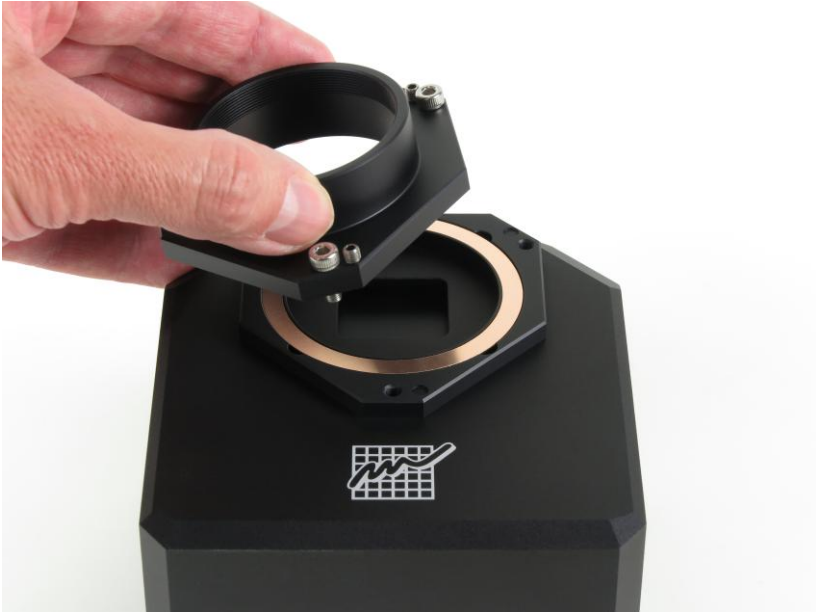
Figure 47: Removing of the adjustable telescope adapter
