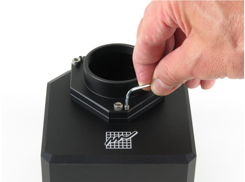
Figure 40: Releasing of the “pushing” screw
