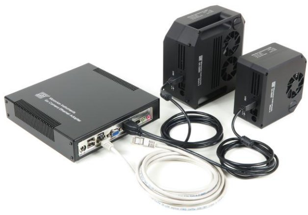
Figure 39: The Camera Ethernet Adapter with two connected cameras
