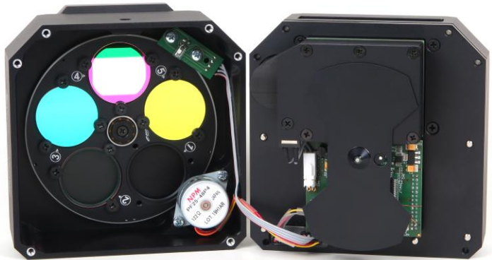
Figure 46: Filters can be exchanged after removing of the camera front cover
