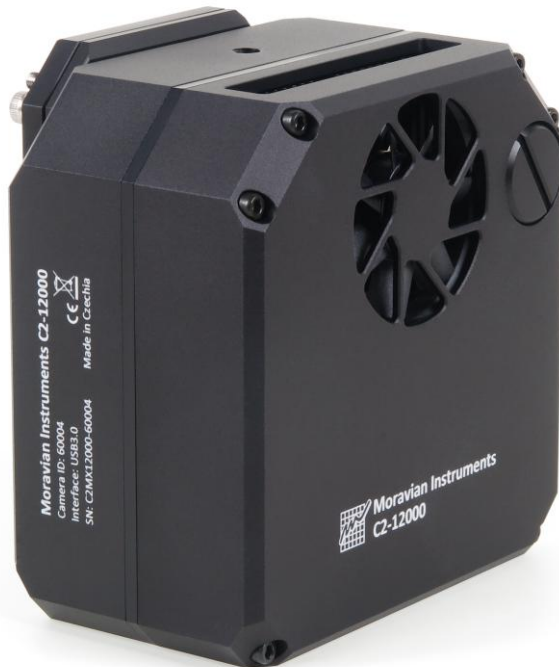
Figure 11: Back side of the C2 camera head contains vents for a fan, cooling Peltier hot side
