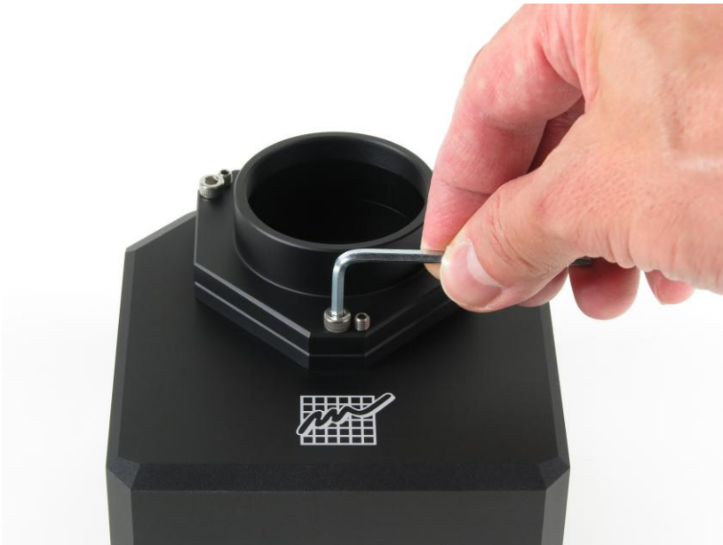
Figure 41: Adjusting of the "pulling" screw
