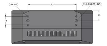
These threaded holes can be used to attach 1.75 inch "dovetail bar" (Vixen standard). It is then possible to attach the camera head, e.g. equipped with photographic lens, directly to various telescope mounts supporting this standard.
