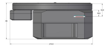
Figure 20: C3 camera head with Enhanced cooling and External filter wheel side view dimensions
