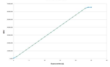
Figure 4: Response of IMX455 sensor in 16-bit mode
