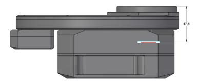
Figure 26: C3 camera with "M" External Filter Wheel back focal distances with  $M68 \times 1$  version 1 adapter
