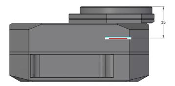
Figure 24: C3 camera with "L" adapter base back focal distances with M68  $\times$  1 version 1 adapter
