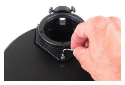
Figure 40: Releasing of the "pushing" screw
