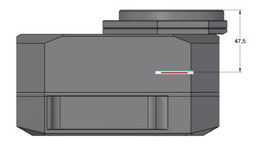
Figure 25: C3 camera with Internal Filter Wheel and "L" adapter base back focal distances with M68  $\times$  1 version 1 adapter
