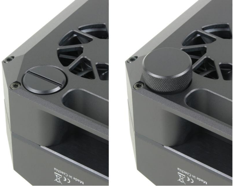
Figure 45: Silica-gel container is accessible from the camera back side
