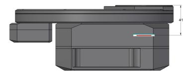
Figure 29: C3 camera with "M" External Filter Wheel back focal distances with M68  $\times$  1 version 2 adapter
