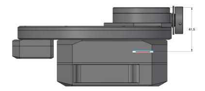
Please note when the OAG has to be used with a camera without filter wheel, it is necessary to use a thick adapter base of the same thickness like the External filter wheel to keep the distance from OAG to sensor constant. Otherwise, the guiding camera cannot reach focus.
