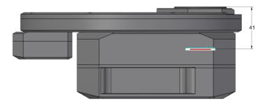
Figure 23: C3 camera with "S" External Filter Wheel back focal distances with short  $M48 \times 0.75$  adapter
