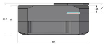
Figure 11: C3 camera head side view dimensions
