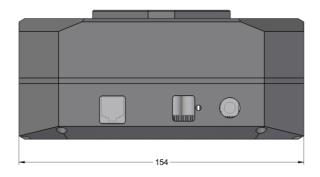
Figure 12: C3 camera head bottom view dimensions
