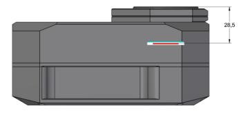
Figure 21: C3 camera with "S" adapter base back focal distances with short  $M48 \times 0.75$  adapter
