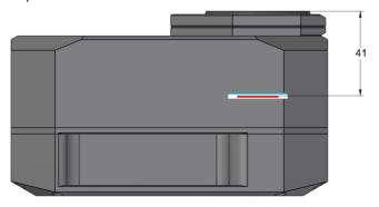
Figure 22: C3 camera with Internal Filter Wheel and "S" adapter base back focal distances with short M48 × 0.75 adapter
