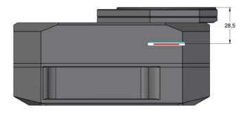
Figure 27: C3 camera with "L" adapter base back focal distances with M68  $\times$  1 version 2 adapter
