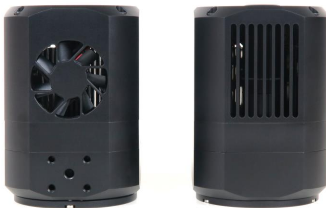
Figure 13: C1× air inlet with fan is on the bottom side of the camera head (left), air outlet vents are on the camera top side (right)
