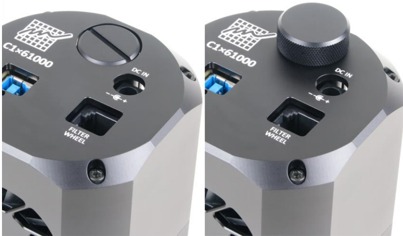
Figure 35: Silica-gel container is accessible from the camera back side
