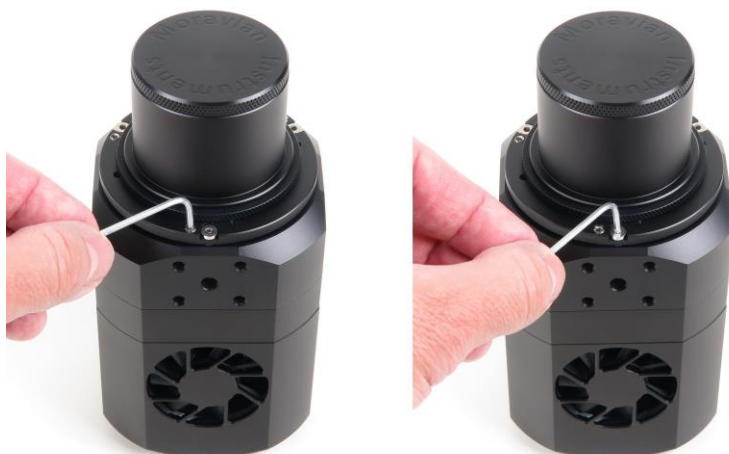
Figure 33: Releasing of the “pushing” screw (left) and adjusting of the “pulling” screw
