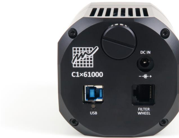
Figure 15: Back side of the C1x camera with the 12 V DC power plug, as well as USB and External filter wheel connectors
