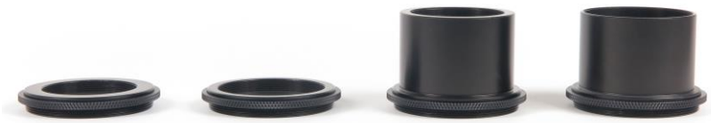
Figure 5: M42 and M48 short adapters with 21.5 mm BFD (left) and long adapters with 55 mm BFD (right) for M56×1 thread
