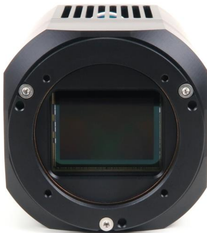
Figure 17: The M56×1 thread and four M3 threaded holes creates the telescope/lens interface of C1× cameras
