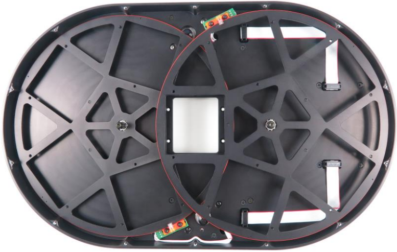
Figure 15: Top and Bottom filter wheels in the SFW shell
