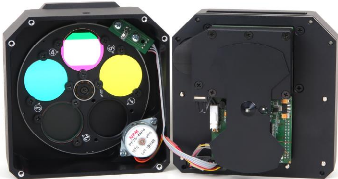
Figure 5: Filters in the Internal filter wheels can be exchanged after removing of the camera front cover
