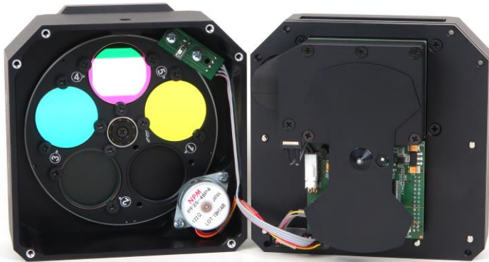
Figure 5: Filters in the Internal filter wheels can be exchanged after removing of the camera front cover
